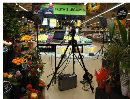
Figure 1. Acquisition of hyperspectral data in the area of fruits in the supermarket.
